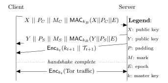
Figure 7: After client and server agreed on the master key  $k_t$  using Uniform Diffie-Hellman, the server is issuing a new session ticket for the client. Afterwards, both parties exchange Tor traffic.
