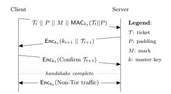
Figure 4: The client redeems a valid session ticket  $\mathcal{T}_t$  containing the master key  $k_t$ . The server responds by issuing a new ticket  $\mathcal{T}_{t+1}$  for future use. After the client confirmed the receipt, both parties then exchange application data.
